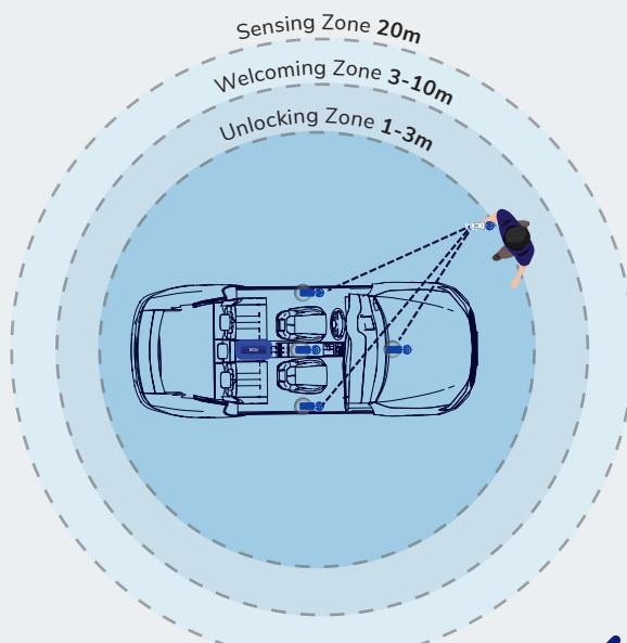
Powered by **high-precision UWB anchors** integrated into the center console and B-pillars, the system enables secure vehicle access using **Time-of-Flight technology**. It is fully protected against relay attacks by accurately verifying the key's true position.
